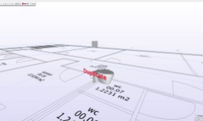
6 . Duplicate components check ... Blake Green Active , Normal 01. Design phase , BIM Model proto...
